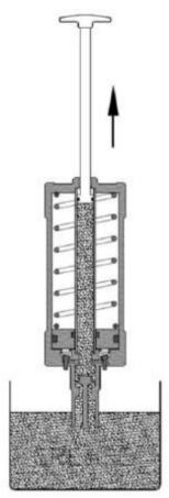
Insert an injection port in the grease and pull the handle up and then wait for 2 seconds.
