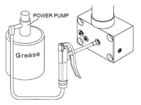
(2) Refill grease by manual grease gun
